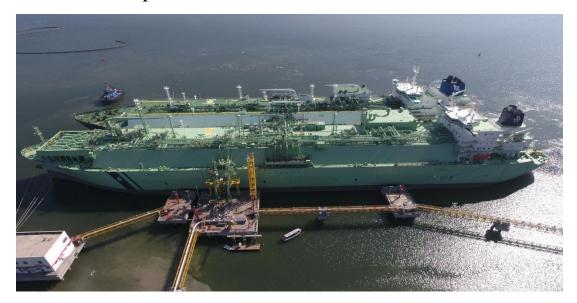
PGPCL operates a brand-new FSRU, BW Integrity, with a storage capacity of 170,000 m3 and peak regasification capacity of 750 mmmscfd. PGPCL is providing services to PLTL in accordance with the operation and Services Agreement (OSA) dated July 1. 2016 and to t5he satisfaction on PLTl. The EPC of the Jetty, owned by PGPCL, was undertaken by Xinjiang Petroleum Engineering Company Limited (XPE) from China.
