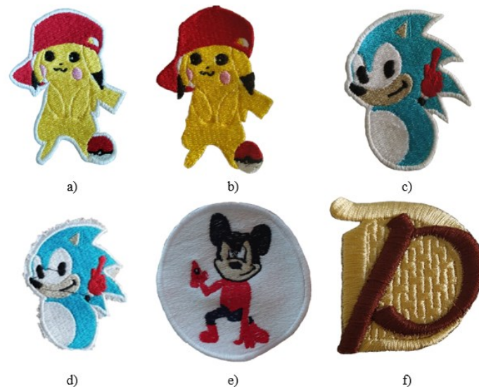
Fig. 7. Samples of embroidered patches: a) standard embroidery with woven fabric with satin stitch row, b) standard embroidery with a woven fabric without satin stitch row, c) standard embroidery with woven fabric with satin stitch row, d) appliqué, e) standard embroidery with two-layers, standard embroidery with nonwoven fabric
